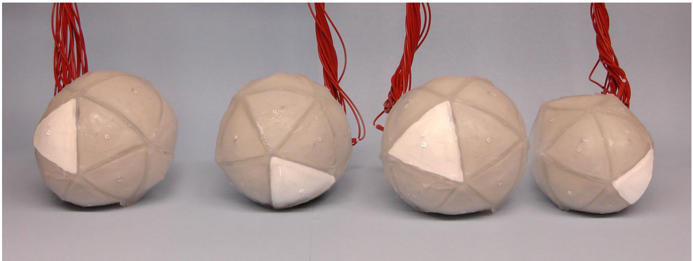
Fig. 10. Composed figures of the JSEL prototype rolling over one revolution. One cell is highlighted to better demonstrate its motion.
